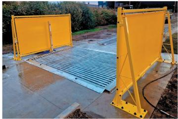
The HydroSan 180 with a draft shield provides protection, improving the quality of disinfection. During high wind, the windshields ensure that the distribution of disinfectant on the surfaces of the vehicle remains even and effective. They also reduce the quantity of solution mist that sprays outside the disinfection area.
